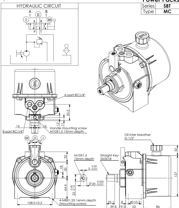
The SBT power pack series is designed for use with horizontal influence drive system by various engines. These power packs have been designed mostly for agricultural use, but can be used in other fields.
